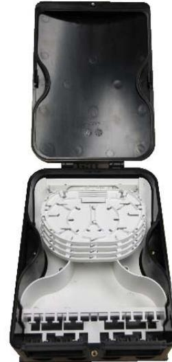
The 24 Customer Pole Mounted Drop Box is designed for use on poles to distribute drop cables to multiple homes. The unit houses four single element splice trays and allows fibres from up to two input cables to be spliced to 24 customer drop cables. All cables enter through the bottom of the box. The box comes with a pole mounting bracket that can be adjusted to meet various pole diameters and is sealed to IP55. The bracket also hides all fixings the pole.
