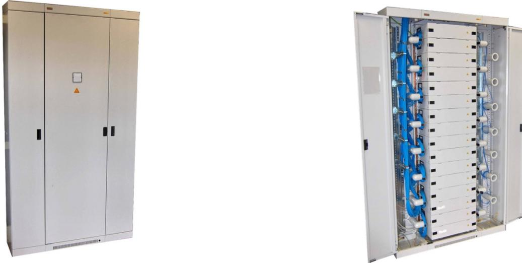
The Modular Main Rack (MMR) is a standard ETSI rack, composed of three independent frames, two Side Channels (left and right) and the Main Frame. The main frame allows the mounting of the Sliding Sub-rack (SSR) series. Three types of Sliding Sub-Rack are available, a Splicing Sub-Rack (SSR-S), a Patching Sub-Rack (SSR-P) and a Splicing and Patching Sub-Rack (SSR-SP).
