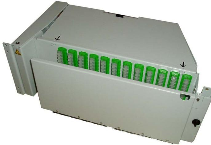
The MEB144 is a 4U left-hand pivoting shelf. It is suitable for mounting into 19" racks or street cabinets. The shelf can splice and terminate up to 144fo within six 24fo splice trays. The unit is supplied with 144 SC/APC pigtailed and adapters, which are pre-installed onto a patch panel.
