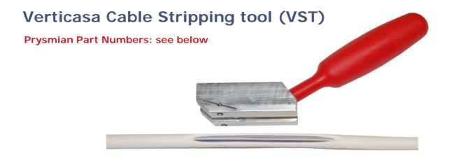
The Verticasa Cable Stripping tool (VCST) is typically used in multi dwelling units or office fibre cabling systems where extractable fibre cables like the Prysmian Verticasa cable range have been installed. It is used to create a longitudinal window cut on the cable. The window cut will allow to access the fibre modules inside the cable.
