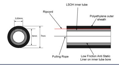
Verticasa Drop Tubes are used to route Verticasa fibre modules to the customers premises. The external drop tube is a 5mm diameter LSOH tube with a low friction liner on the inside wall of the tube, over-sheathed with a polyethylene sheath to provide weather resistance and protection from UV light. The internal tube also contains a pre-installed pulling rope to make fibre installation easy.
