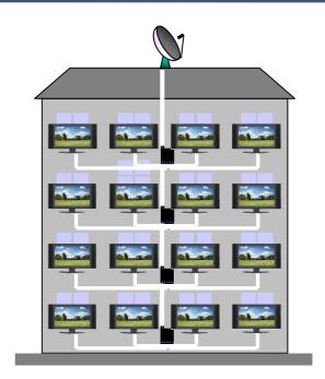
VerTV<sup>™</sup> is an optical multi dwelling unit TV cabling solution. The plug and play solution consists of patchcords of various lengths and floor boxes for splitting or tap off. It has been designed to make installation simple as no fibre optical experience is required for installation, as no fusion or mechanical splicing is needed. The splitter and tap off boxes are simply connected together using patch-cords, which utilise a push fit small form connector.
