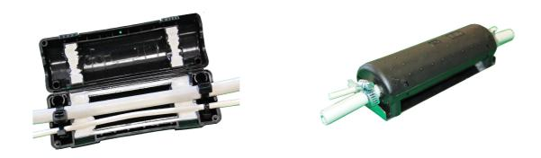
The Outdoor Verticasa Breakout unit is used to breakout and distribute the fibres from an in-line Verticasa cable into drop tubes, for routing to a customer premises. It is UV resistant and sealed to IP67, enabling it to be mounted in the outdoor environment. It has the capacity to accommodate an in-line Verticasa cable of up to 13mm in diameter. It enables a window to be cut in the cable to access the fibres, which can be spurred of into a drop tube of up to 7.2mm in diameter.
