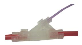
The Mini Branch Connector is a small single piece snap fit closure. It is used to join a 7mm duct and enable retracted fibres to be spurred off into a 4mm branch duct. The unit is used to connect the ducts mechanically and does not offer any protection against the ingress of water. The Connector is supplied as a pack of 10 pieces.
