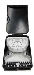
The 24 Customer Pole Mounted Drop Box is designed for use on poles to distribute drop cables to multiple homes. The unit houses four single element splice trays and allows fibres from up to two input cables to be spliced to 24 customer drop cables. All cables enter through the bottom of the box. The box comes with a pole mounting bracket that can be adjusted to meet various pole diameters and is sealed to IP55. The bracket also hides all fixings the pole.
