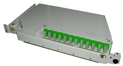
The POB36 is a 1U left-hand pivoting shelf, suitable for mounting into 19" racks or street cabinets. The shelf can splice and terminate up to 36fo within three 12fo splice trays. The unit is supplied with 36 SC/APC type pigtails and adapters, which are pre-installed onto a patch panel.
