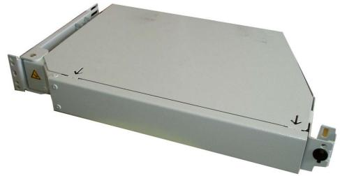
The MOE96 is a 1.5U left-hand pivoting shelf, suitable for mounting into 19" racks or street cabinets. The shelf can splice up to 96fo within twenty four 4fo splice trays. Up to six 5mm tubes or cables and one 11.5mm cable can be installed into the shelf.
