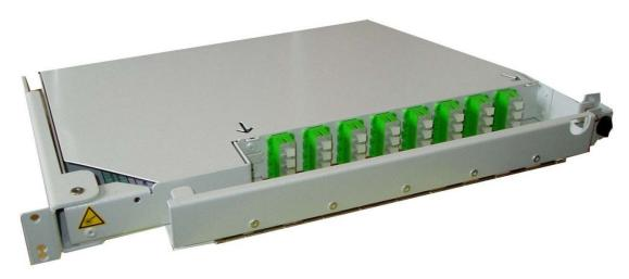
The MEC32 is a 1U Pivoting shelf, suitable for mounting into 19" racks and street cabinets. The shelf can accommodate up to eight 1x4 or four 1x8 or one 1x32 pre- terminated splitters. The shelf is supplied with SC/APC adapters and splitters pre-installed.
