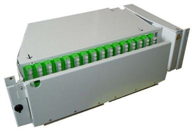
The MEC128 is a 3U Pivoting shelf, suitable for mounting into 19" racks and cabinets. The shelf can accommodate up to four 1x32 or two 1x64 pre-terminated splitters. The shelf is supplied with SC/APC adapters and splitters pre-installed.
