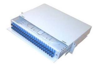
The DOBEX-2U Distribution Drawer is a 2U splice and patch panel for installation into 19" or ETSI racks. The product is fully metallic and has a capacity of up to 96 fibres on a splice and patch basis. The product can be configured with FC, ST, E2000, SC or LC type pigtails and adapters..
