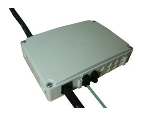
The Riser Box is designed for use within apartment blocks and mid/high rise office blocks. The unit houses a single integral splice tray, and allows fibres from an in-line or butt Blown Fibre tube cable to be spliced up to 12 customer drop cables. In cases where Blown Fibre tube cables are to be used for the customer drops, bulkhead tube connectors can be fitted to the unit.
